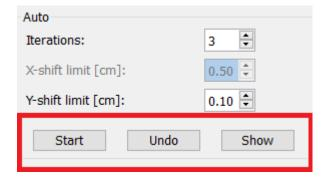
Press "Start" to initiate an automated motion correction. A "HybridRecon-MoCo" window will appear when the motion correction is finished. A visual representation of the motion correction changes, made to your MoCo projection, will be shown in this window. You may compare your original projections to your MoCo projections SPECT using the media buttons.
