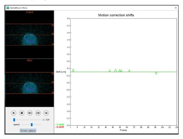
The "Man" section will be available if the "Moco type" is set to manual ("Man"). Your projection may be moved using the arrows. If the "One frame only" radio-button is toggled on, the change will be applied to only one frame. You may use the media buttons, the sliders or the mouse wheel (if your cursor is over the cine picture), to change the projection.
