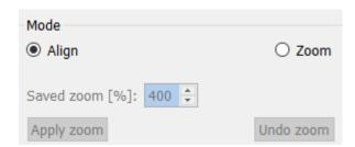
In the "Align" mode, dotted crosses will be displayed over your TCS views. You may move the cross over your SPECT by using your mouse. Each of your TCS views will automatically triangulate over the new cross location. Two options are available for rotating your views: slide the mouse to the required angle on the scale below your TCS views, or change the value in the right scale field. To alter a value, either type it in or use the up and down arrows.
