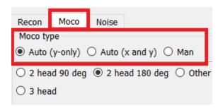
The "Auto" section will be available if an automatic motion correction type is selected. The "Start" button allows you to perform an automatic motion correction. The "Undo" button restores the original projections. The "Show" button allows you to display the "MoCo" box. When no motion correction has been applied, this button is greyed out.
